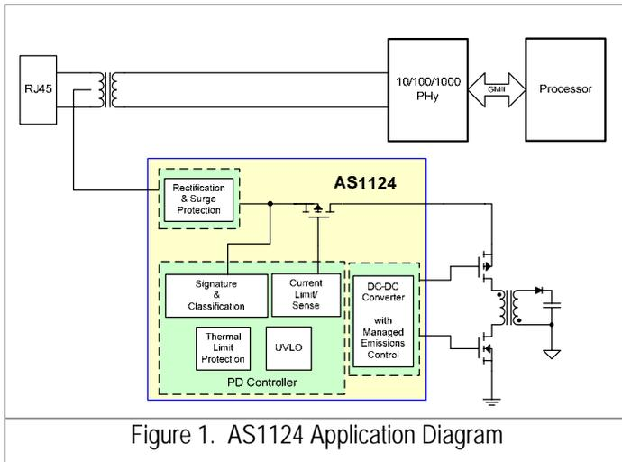
Figure 1. AS1124 Application Diagram
