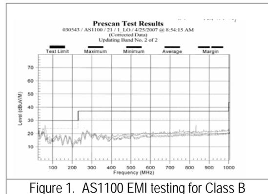
Figure 1. AS1100 EMI testing for Class B
